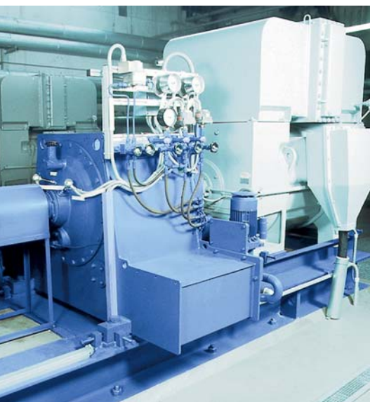
Variable-speed turbo coupling type SVTL in boiler feed pump drive.
