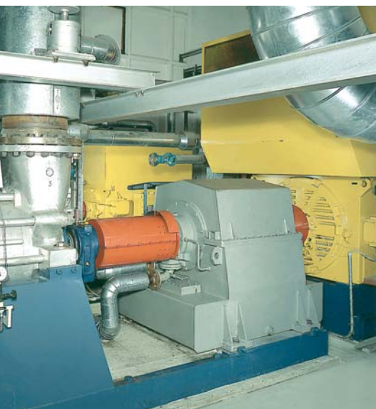
Variable-speed turbo coupling type SVNL in circulation pump drive.
