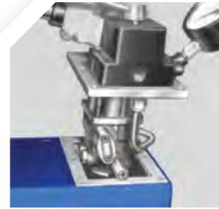
**4008** – Hydraulic hand pump with No. 9584 2-position, 3-way control valve (for operating single-acting rams), and No. 4006 BL2 2-gallon reservoir with legs.
