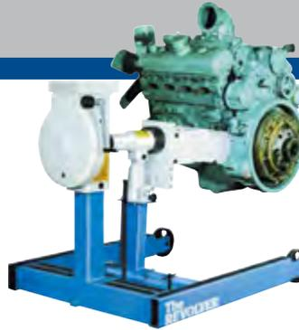
**1750A** – Revolver diesel engine stand with No. 205061 universal engine adapter assembly.
