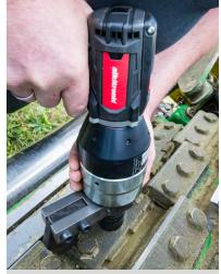
Repeat shut-off accuracy ± 3% (same bolting connection). All *alkitronic*<sup>®</sup> torque multipliers are CE-certified.
